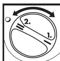
**Machines with 2-speed gear units (Xo4R/Xo6)** have two maximum speeds available (First gear: Slow / Second gear: Fast).
