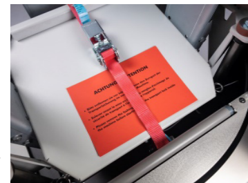
Transport lock with lashing belt
