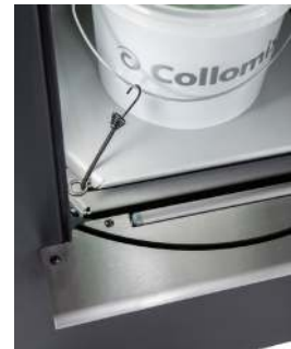
Securing the handle with a rubber band
