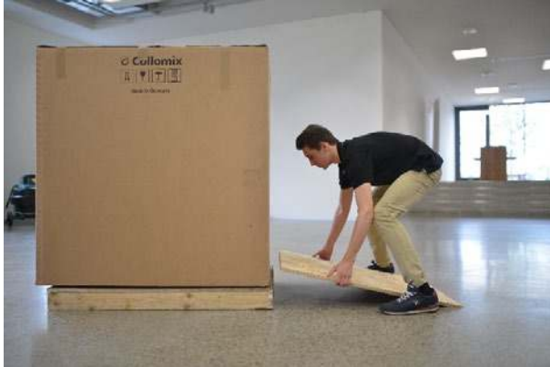
Figure 10 Detailed view, putting the ramp in position
