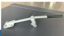
Always use the handling tool to remove metal containers from the biaxial mixer ROTA 400 and ROTA X.40. If you do not have a handling tool, please contact your service contact for mixers and shakers.
