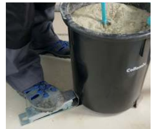
Only press with your foot: Secure fixation without forced posture
